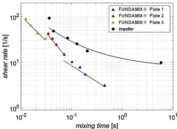
Figure 3: A FM-1 with type A plates of diameters 22, 45, and 65 mm was tested at 100 Hz and amplitudes of 1, 1.5, 2, and 2.5 mm. The data was compared with a 4-blade glass impeller (IKA) with 29 mm diameter, running at 50 – 2'000 rpm [2].
