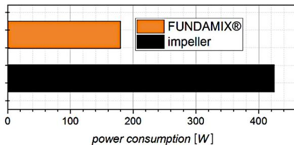
Figure 2: The same FUNDAMIX® and impellers were used as in Fig. 1, running at an amplitude of 2.3 mm and a rotational speed of 500 rpm, respectively [1].
