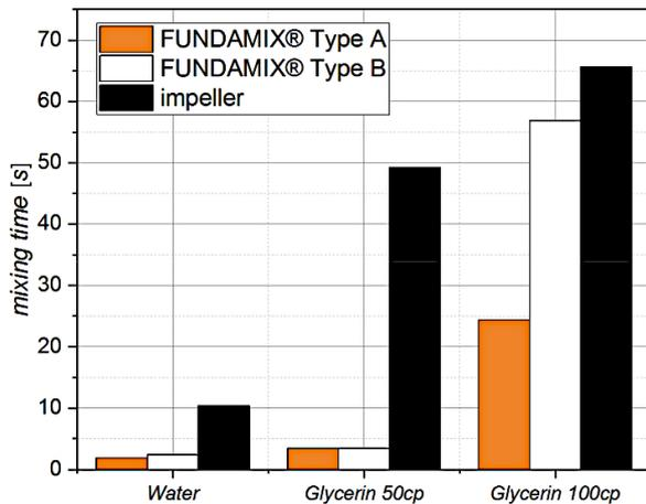
Figure 1: A FM-2 with a 135 mm diameter plate was used, running at a 2.3 mm amplitude and 100 Hz. The data was compared with the average mixing times of a two-blade Ekato Isojet and a 3-blade Lightnin A310 impeller, both having a 132 mm diameter and running at 500 rpm [1].
