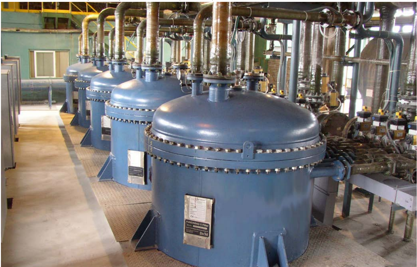
5 FUNDABAC® filters, each 47 m 2 area, vessel carbon steel, hard rubber lined, ø 1900 mm, internal components PVDF, for the filtration of viscose fibres, yield per cycle 1.5 to solids of 70% dry substance
