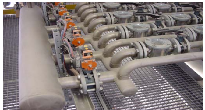
Fig. 3: Filtrate outlets including sight glass and manual shut-off valves for each outlet. Outlets are grouped into headers with individual pneumatically actuated valves leading into the filtrate collector.
